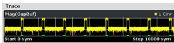
Fig. 9-7: Preview of capture buffer
